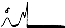
Fig. 3. Ascending pattern at pH 2 of the fraction soluble in alcohol in the presence of 0.167 M sodium chloride.
